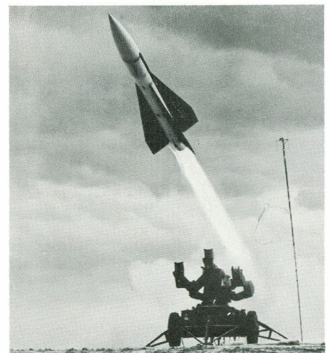
The Army's HAWK missile here leaves its three-place launcher to intercept a target plane. Homing all the way, the HAWK is a particularly effective air defense weapon. Developed by Raytheon Manufacturing Company, it is now in production at Raytheon's plant in Andover, Mass.
